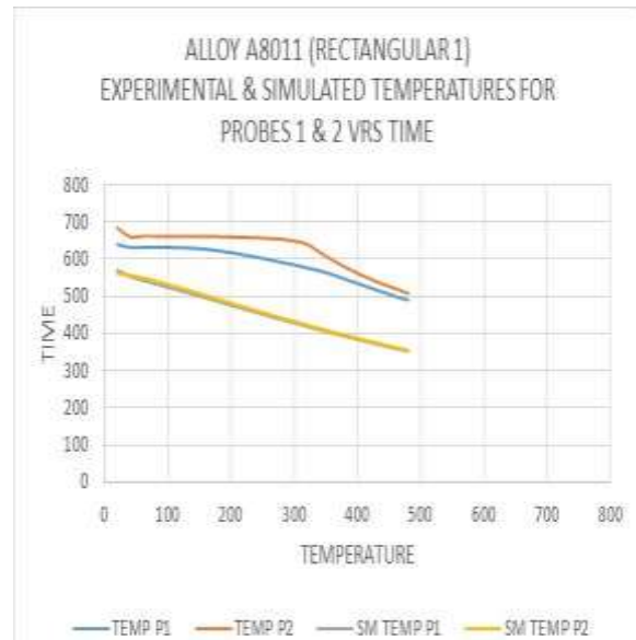
Fig. 9: Probe 1 and 2 temperature profile (experimental and simulated) for Alloy A8011 (Rectangular 1)
