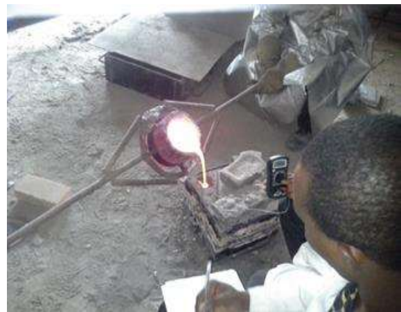
Fig. 6: Liquid metal being poured into one of the moulds
