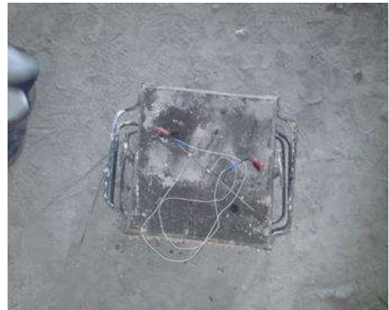
Fig. 5: Prepared and coupled mould with thermocouple probes
