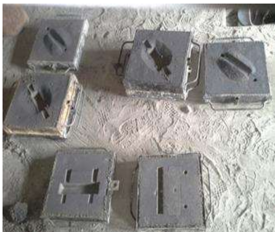
Fig. 4: Mould for one of the rectangular shapes
